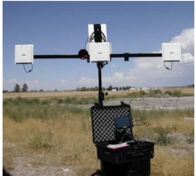
The HAZMAT CAM viewing console and true diversity receiver. The three-antenna, true diversity receiver minimizes signal distortion in urban environments.
