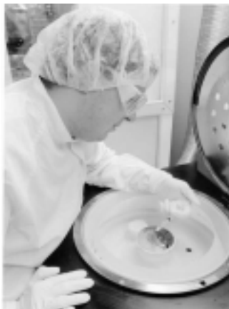
Scientists dispense a solution on a bare silicon wafer inside a spin coating device (shown here) during the development of thin films for improved semiconductor materials.
