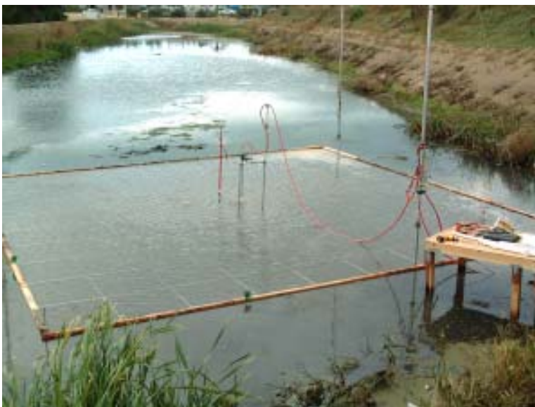
Demonstration of ADAS Air Sparging Technology
